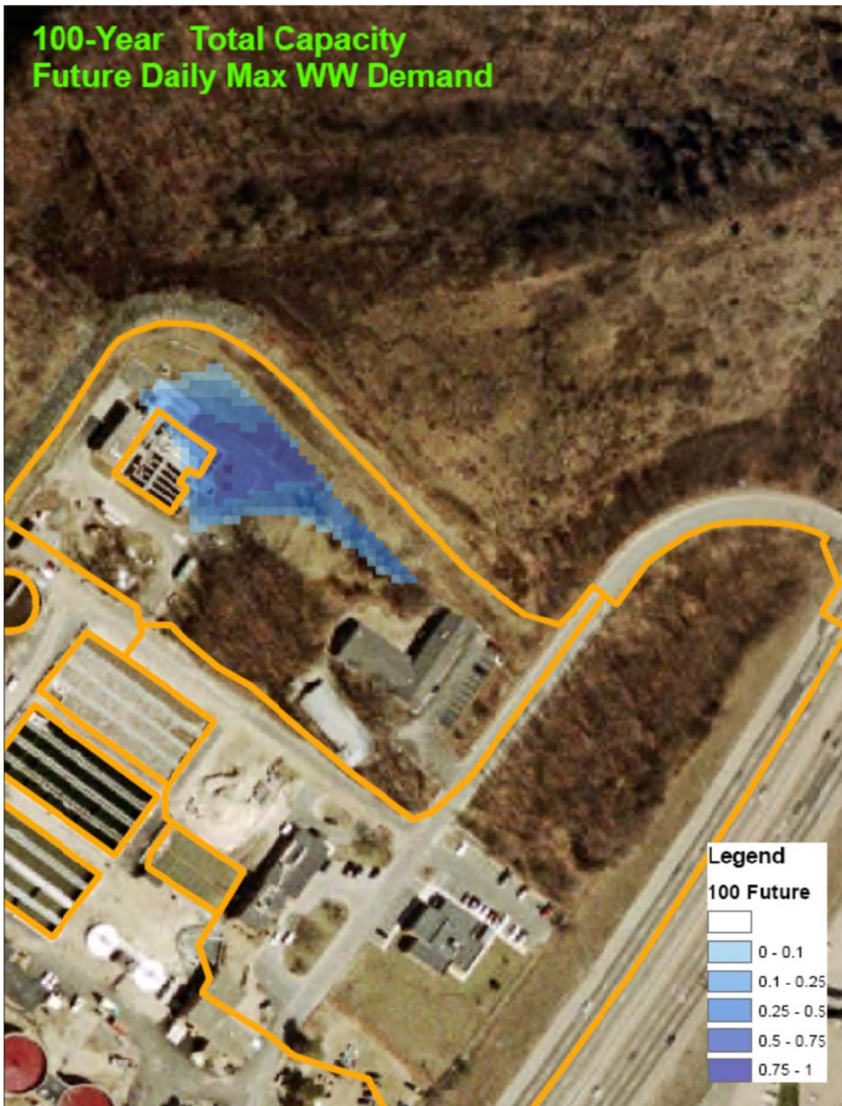
Figure VI-4: 100-year Future Day Flood Area – Total Capacity
