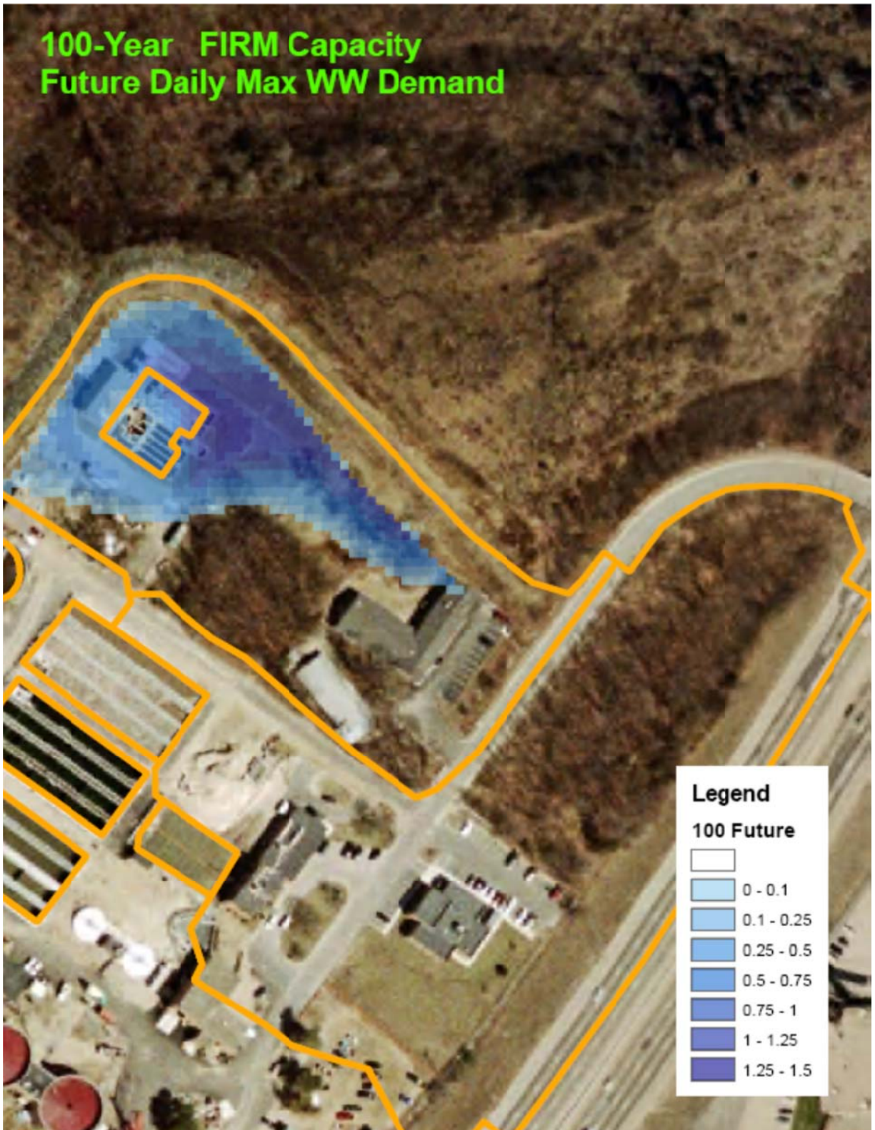
Figure VI-3: 100-year Future Day Flood Area – Firm Capacity
